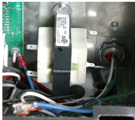
Figure 3: Reposition the 12-volt transformer in the spot occupied by the removed 24-volt unit. Shown with wires removed for clarity.
